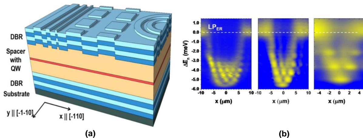
Figure 1 (a) Schematic overview of a structured microcavity. The blue layers depict the DBR, the yellow layer depicts the spacer layer and the red layer depicts the quantum well structure. (b) Confined LP energy states in non-etched wire mesas with a width of  $w=10\mu\text{m}$  (left),  $w=6.4\mu\text{m}$  (center) and  $w=3.2\mu\text{m}$  (right).  $LP_{ER}$  depicts the reference energy, which is the LP energy in the etched area.
