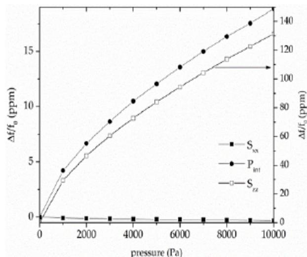
Figure 2: The  $\overline{S_{xx}}$ ,  $\overline{S_{zz}}$ ,  $\overline{P_{int}}$ -induced ZGVR relative frequency changes versus the applied differential pressure for the 1–1 composite plate.
