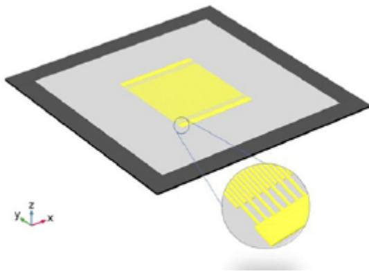
Figure 1: The schematic of the suspended membrane: the silicon frame is black, the membrane is gray; the IDT is yellow.
