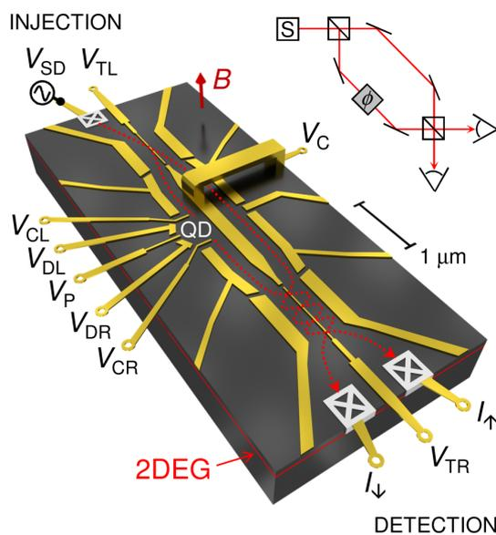
Figure 1: Schematic of our electron interferometer showing surface electrodes defining the conductive channels (red, dotted lines) in the two-dimensional electron gas (2DEG) located below the surface.
