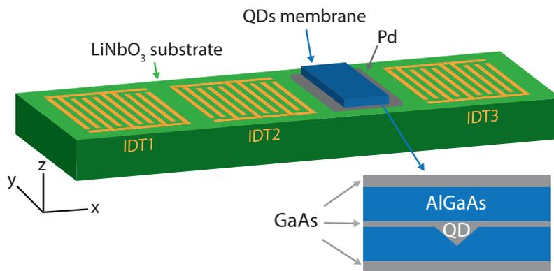
Figure 1: Schematic of the hybrid device composed of a QD membrane transferred by epitaxial lift-off on a LiNbO<sub>3</sub> SAW-chip patterned with two delay lines. A schematic of the QD heterostructure is shown in the lower part.
